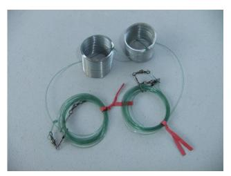
The end result is that this portable dipole expands to 18.5'L from its collapsed state of only 2.5"L, and works just great for the travelling Ham.
